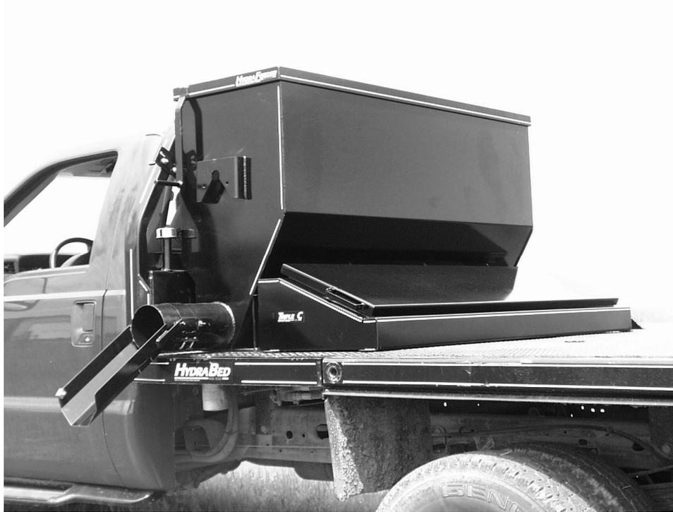
*Hydraulically Powered Supplement Feeder*
